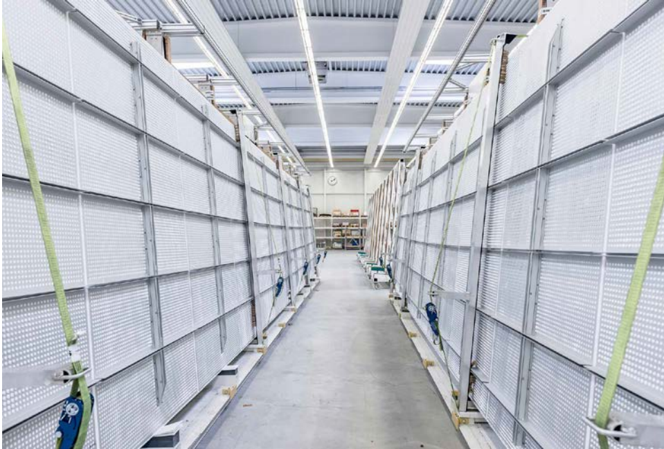
Composite system of glass and silicone-glued aluminium cassetts. ©seele/René Müller
