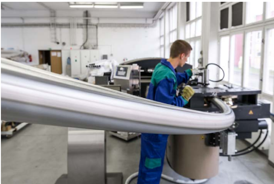
Self-learning machines for bending and measuring the stainless steel tubes. ©seele/René Müller
