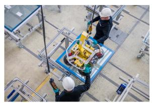
High degree of flexibility at seele in Gersthofen: rotary assembly tables for assembly developed especially for a project. ©seele
