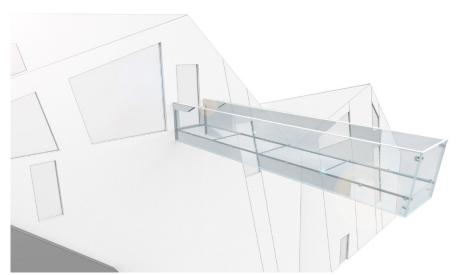
Visualisation of the glass walkway made of low-iron glass. The special connection to the existing building enables maximum transparency. © seele
