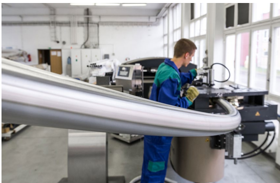
3D tube-bending machine processing stainless steel tubes for the King Abdulaziz Center for World Culture © seele/René Müller
