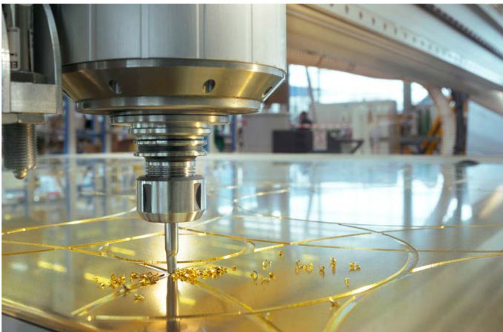
Milling of ornamentals at seele's production in Gersthofen/Germany © seele/Bernd Müller
