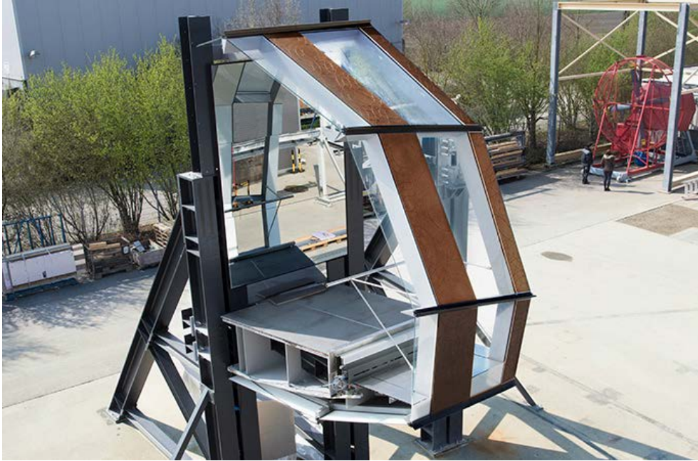
The mockup construction at the seele test site in Gersthofen presents a vertically halved section of the CF TEC Bridge of 3m in length. ©seele
