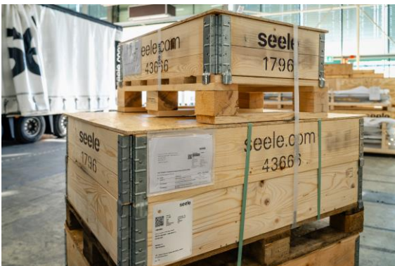
The RFID transponder (bottom) with a titanium chip on the back complements the traditional delivery slip (top) on every packaging unit. © seele
