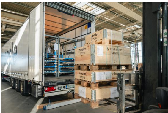
Every packaging unit has its own RFID label on the long side so that it can be detected by the reader device. © seele
